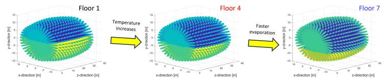
Level of whiskey in barrels on different floors after 20 years of simulation time (whiskey, air gap, unsaturated staves, saturated staves)
